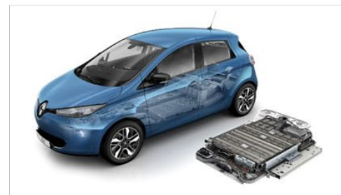
Renault Zoé 400 V, 41 kWh, 12 modules, 192 cellules, 290 kg
